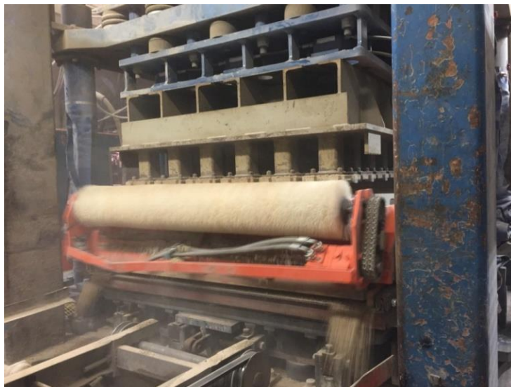
Figure 12: First step of paver manufacturing cycle
