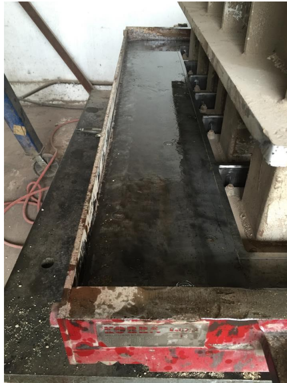
Figure 18: A cleaned mold surface
