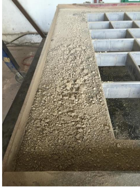
Figure 19: Debris formed on mold surface due to material accumulation
